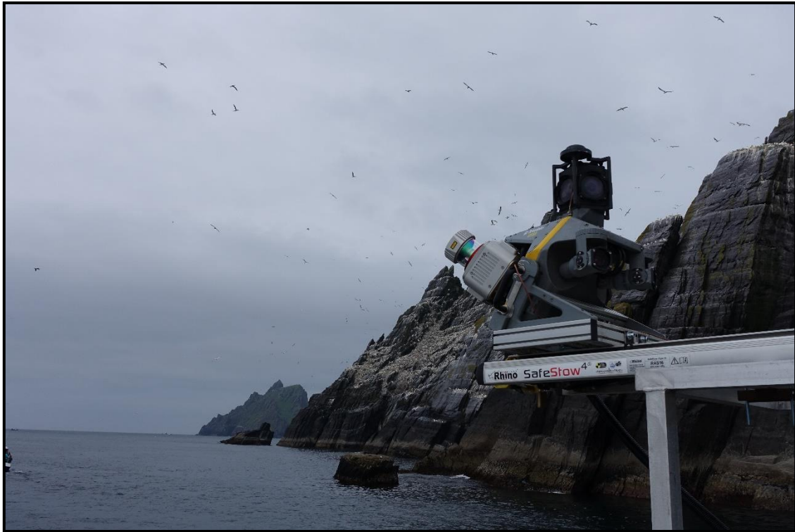
Figure 9 Hull mounted laser scanner on INFOMAR's survey vessel RV Keary undertaking a survey of both islands.
