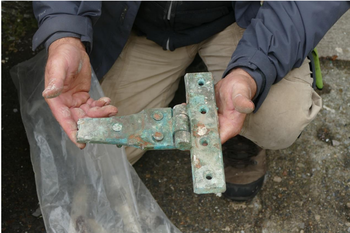
Fig. 21. – Original bronze hinge from Upper Lighthouse buildings
